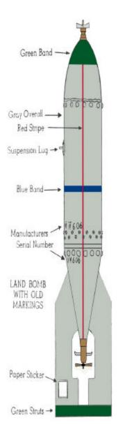
One fin is missing and fin is offset 45 ° for clarity
