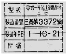
Main fuselage data stencil from Zero 3372. The first line reads: Type Zero No.1 Carrier Fighter Plane Model 2. The second line reads: Mitsubishi Dai 3372 No. The third line is the date of manufacture: 1941/October/21. Photo courtesy Don Marsh via j-aircraft.com
