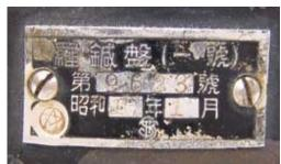
Japanese KI-21 Sally Bomber compass MK 1 model 2 data plate. This type of compass was fitted above the instrument panel in Sally bombers of the Imperial Japanese Army. The data plate has an Army Star stamped on it. The data plate shows that the serial number is 9623 and the date of manufacture was January and the year was in the Emperor's Reign Showa 16 – this being 1941. Photo www.warbirdsite.com
