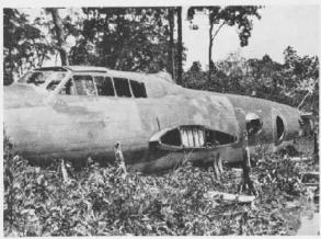
3 With wings and tail surfaces removed, fuselage of Betty lies in swamp, ready for the big job of moving it to tidewater for reshipment; Betty is Japan's fastest bomber, carrying five to seven men at speeds up to 288 mph, flying as high at 29,000 ft.
